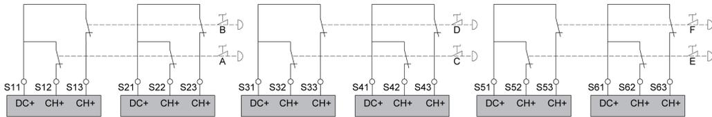
Wiring of the inputs for guards
