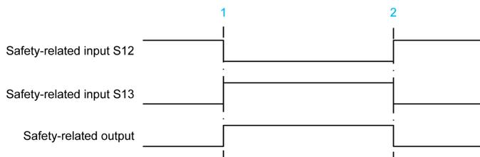
1 = Activation, transition to operating state Run: Outputs Energized
