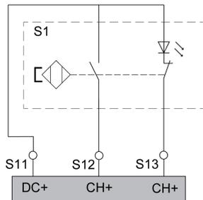
If the level at terminal S12 is logically 0 and the level at terminal S13 is logically 1, the safety-related input is activated.
