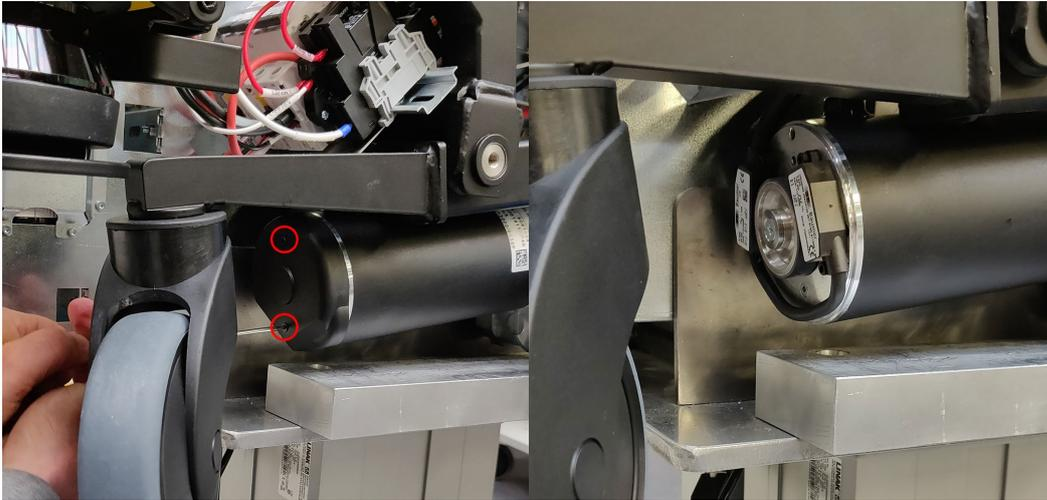
3. Verify that the encoder cables are still intact and positioned correctly so they are not in contact with the magnetic wheel. If the cable is worn down, you must replace the bogie with the faulty cables. See the guide *How to replace the bogie with motor on MiR100/MiR200*.
