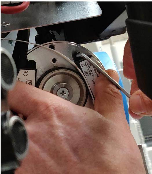
7. Repeat steps 5 and 6 with the second encoder, and put the cap back on. Once you have adjusted the second encoder, ensure the encoder cable is placed along the edge of the motor.
