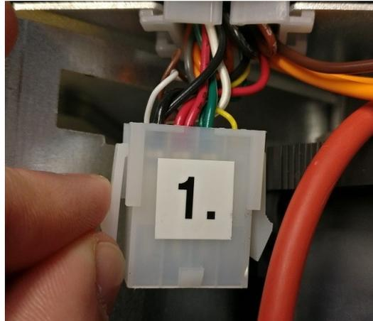
2. Do not unplug the connector. The image above is intended to be used to identify the connector. If the connector has a black shrink tube, cut it away to access the pins.
