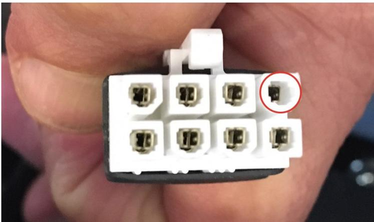
5. After checking all crimps and fixing any faulty ones, reconnect the encoder connectors gently.
