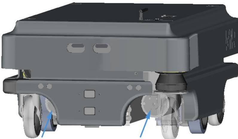
2. Use the T20 Torx key to unscrew the two screws located on the encoder cap.
