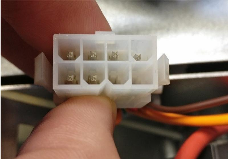
3. Use a small thin tool, such as a screw driver, to try to push the crimp back into place. The crimp should click into place when positioned correctly.
