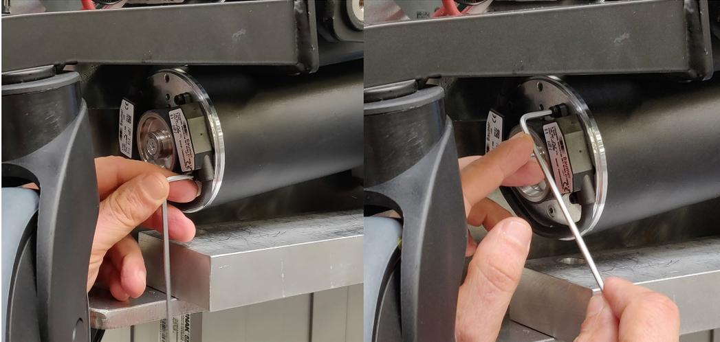
6. Place the 0.3 mm thickness gauge between the encoder and the magnetic disk. Push the encoder with one hand against the gauge, and screw the bolts back in to fix the encoder in place.
