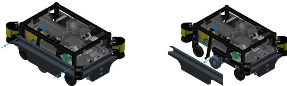
Each motor contains two encoders, so there are four encoders in total that can be faulty. The encoders are located right behind the front caster wheels on both sides of the robot.
