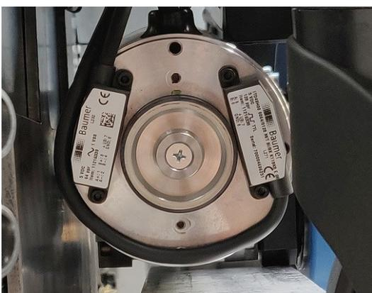
5. Use hex key 2.5 mm to unscrew the two bolts on one of the encoders. Once the encoder is removed, apply Loctite 2400 threadlocking adhesive or similar adhesive to the encoder mounting holes, and place the encoder back in its original position.
