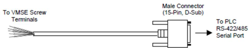
Figure 30 Wiring Diagram
