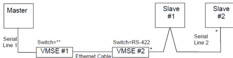
\* Termination is required across RD or RX terminals at these locations if the serial line is greater than 6 feet (2 meters) long
