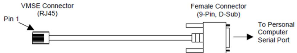
Figure 28 Wiring Diagram
