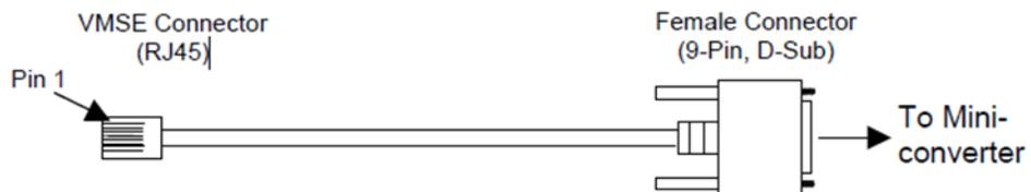
Figure 26 Wiring Diagram
