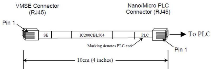
Figure 24 Wiring Diagram for IC200CBL504
