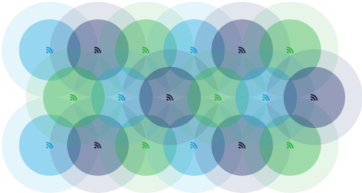
Figure 4.1. Illustration of a simplified scenario where access points cover a circular area in a site without any interference from structures or other devices. In this case three WiFi channels are used, and the access points are configured so there is the greatest distance possible between access points on the same channel.
