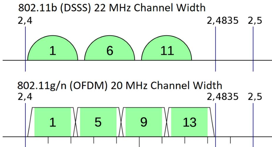
Figure 4.2. Channel separations on 802.11b and 802.11g/n standards.
