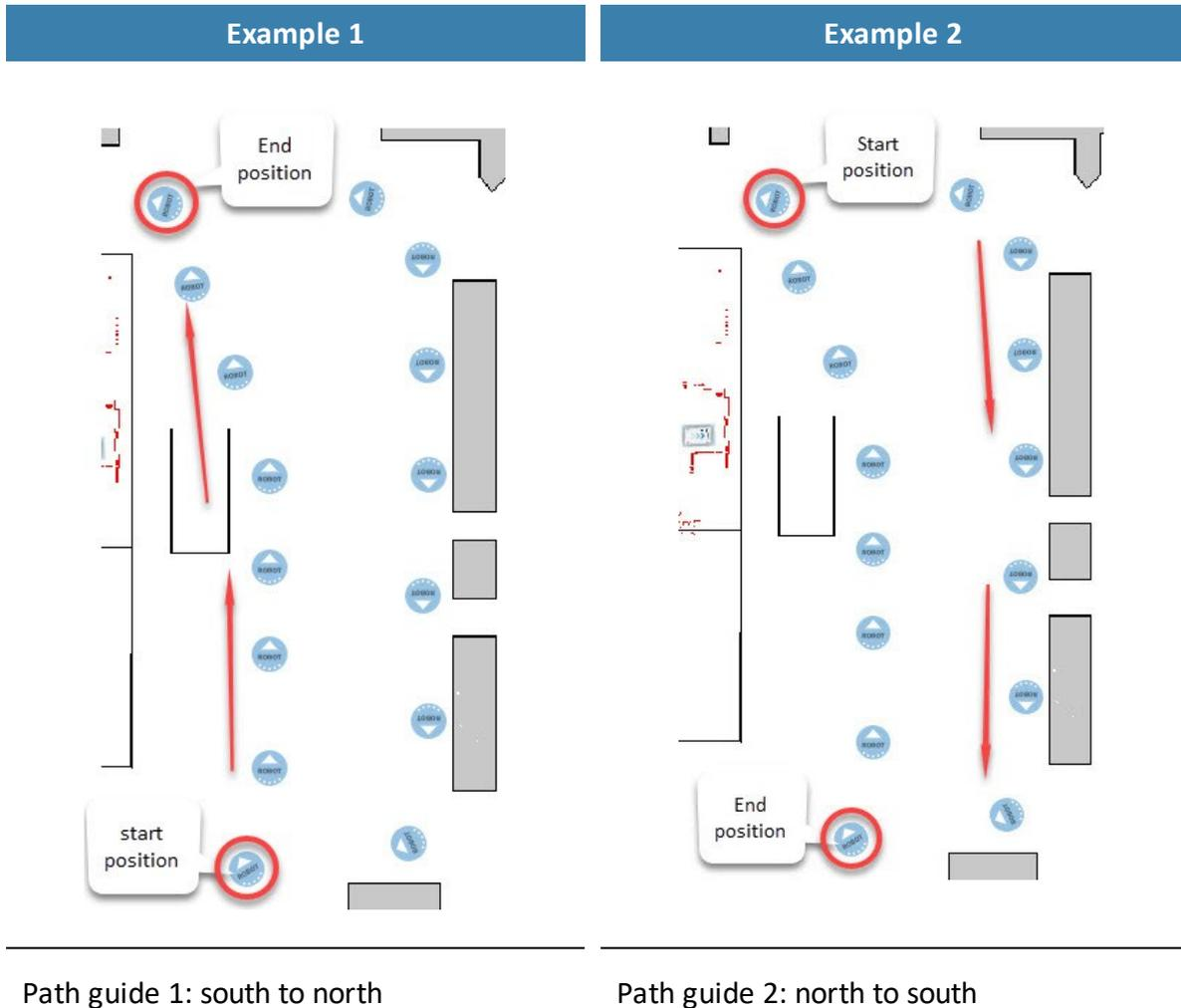
Path guide 1 forces the robot to follow one lane going south to north, and Path guide 2 forces the robot to follow another lane going north to south. The same two positions are used for start and end positions but reversed in the two path guides.
