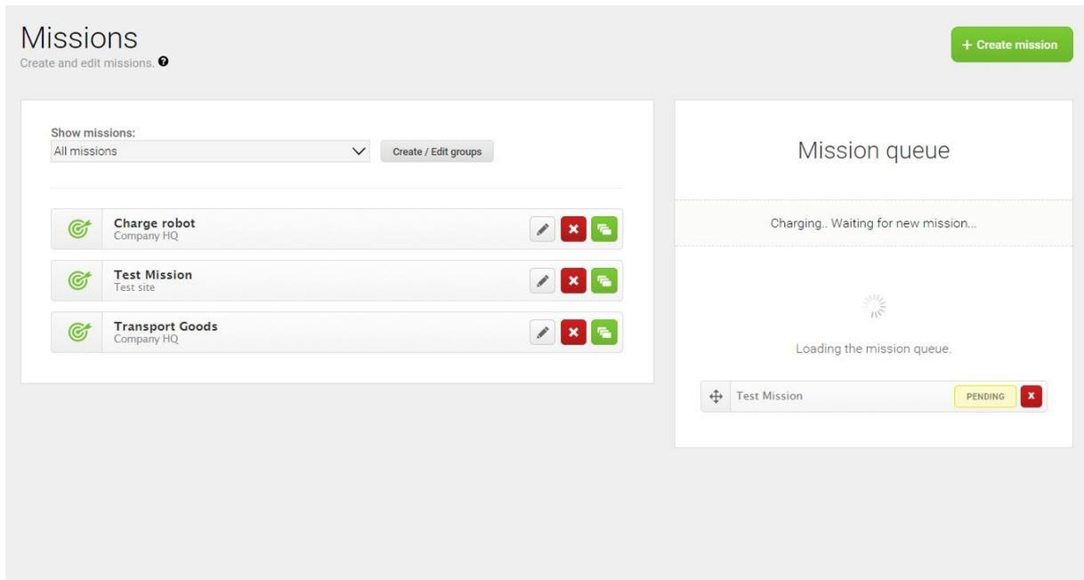
If there are variable parameters in a mission, for example a variable position, you will be asked to select the position when adding the mission to the queue.
